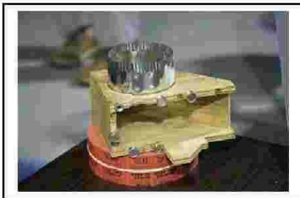
John Marsh made this dust extractor for his Delta saw. It is held in place by magnets.
