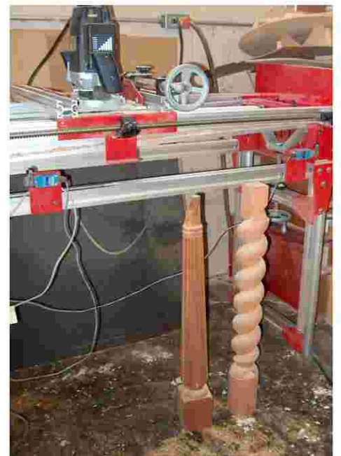
Spiral & Fluted legs made on the Legacy machine
