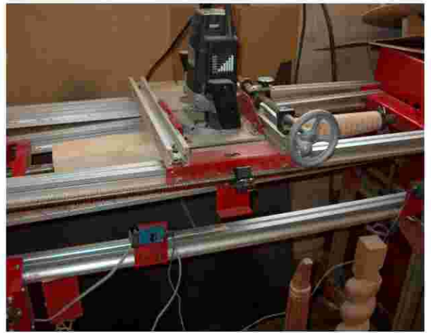
Spiral & Fluted legs made on the Legacy machine
