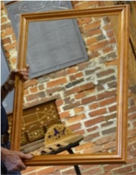
Palmer Burke made this stunning frame out of cherry. He used three different router bits to create the unique profile. This has a lacquer finish.
