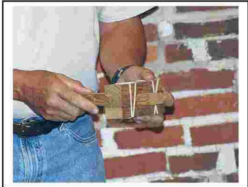
Andy Obin shows how to make shelf bracket using keyhole hooks. Andy also showed how he makes mallets by cutting and gluing together several pieces of wood. The mallet shown was made from Teak.
