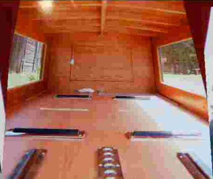
Palmer Burke brought in photographs of the hearses he has built for use with a motortrike. These are constructed on an aluminum frame of oak and MDO plywood. They are for sale and listed in a national magazine.
