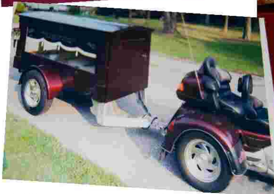
Palmer Burke brought in photographs of the hearses he has built for use with a motortrike. These are constructed on an aluminum frame of oak and MDO plywood. They are for sale and listed in a national magazine.
